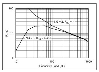
FIGURE 13. Required R<sub>s</sub> vs Noise Gain.
