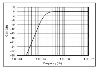
FIGURE 9. Frequency Response for the Filter in Figure 8.
