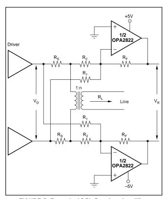
FIGURE 5. Example ADSL Receiver Amplifier.
