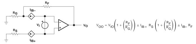
Figure 25. Output Offset Voltage Model
