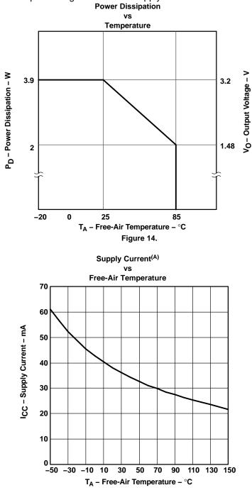
A. Data Transfer = 30 MHz / All Outputs, ON/V<sub>O</sub> = 1 V / R<sub>IREF</sub> = 600  $\Omega$  / AV<sub>DD</sub> = 5 V Figure 15.
