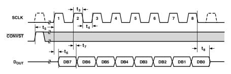
Figure 16. Serial Interface Timing
