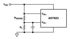
Figure 9. DC Current Measurement Scheme
