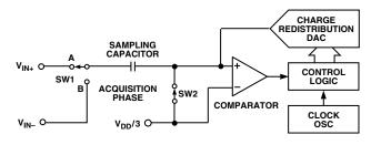
Figure 4. ADC Acquisition Phase
