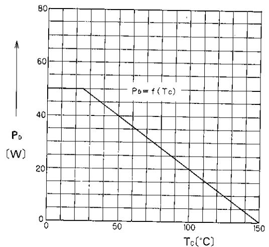
Allowable Power Dissipation vs.  $T_c$
