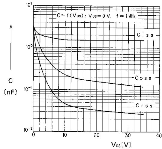
Typical Capacitance vs.  $V_{DS}$
