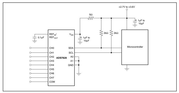
FIGURE 1. Simplified I/O of the ADS7828.
