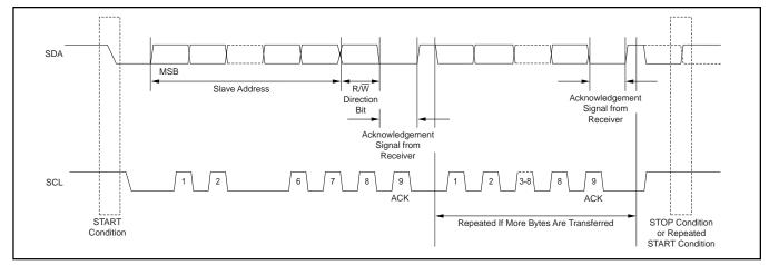
FIGURE 2. Basic Operation of the ADS7828.
