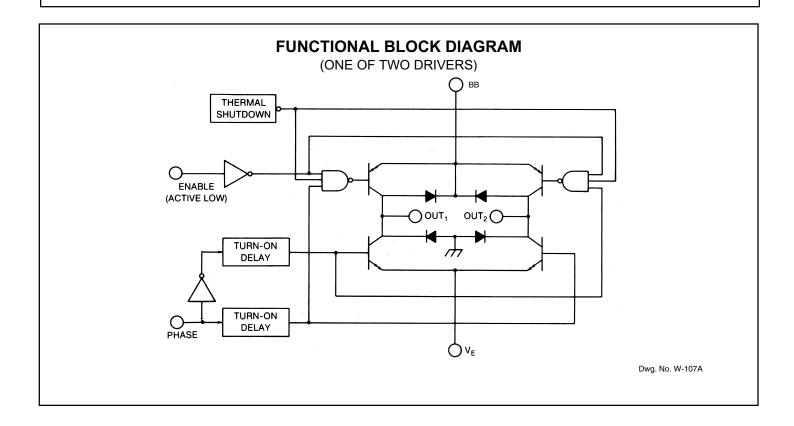
To maintain isolation between integrated circuit components and to provide for normal transistor operation, the ground tab must be connected to the most negative point in the external circuit.
