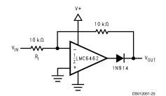
FIGURE 19. Full-Wave Rectifier with Input Current Protection (R<sub>I</sub>)
