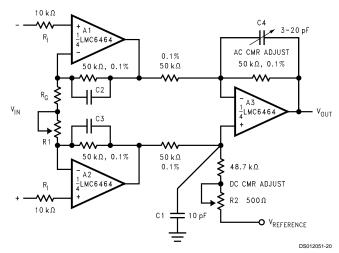
FIGURE 14. Low Power Three Op-Amp Instrumentation Amplifier
