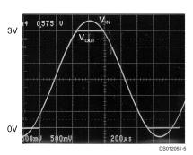
FIGURE 1. An Input Voltage Signal Exceeds the LMC6462/4 Power Supply Voltage with No Output Phase Inversion
