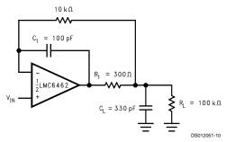
FIGURE 6. LMC6462 Non-Inverting Amplifier, Compensated to Handle a 300 pF Capacitive and 100  $k\Omega$  Resistive Load
