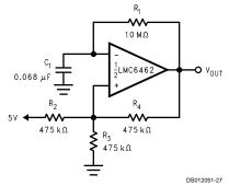
FIGURE 21. 1 Hz Square-Wave Oscillator
