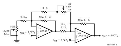
FIGURE 15. Low-Power Two-Op-Amp Instrumentation Amplifier
