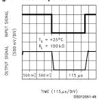
Non-Inverting Large Signal Pulse Response
