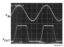
FIGURE 2. A ±7.5V Input Signal Greatly Exceeds the 3V Supply in *Figure 3* Causing No Phase Inversion Due to R<sub>I</sub>
