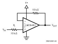
FIGURE 18. Half-Wave Rectifier with Input Current Protection (R<sub>I</sub>)
