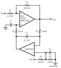
FIGURE 22. High Gain Amplifier with Low Frequency Null
