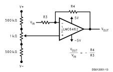
FIGURE 9. Inverting Configuration
