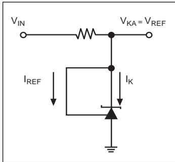
Figure 2. Test Circuit for V<sub>KA</sub> = V<sub>REF</sub>
