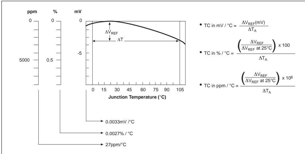
Figure 1. V<sub>REF</sub> VS Temperature.
