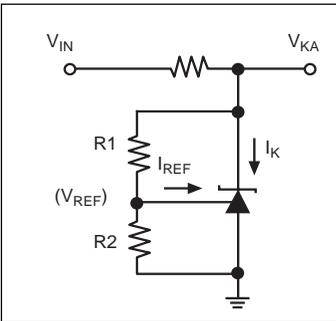
Figure 3. Test Circuit for V<sub>KA</sub> > V<sub>REF</sub>
