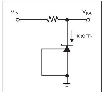
Figure 4. Test Circuit for I<sub>KOFF</sub>
