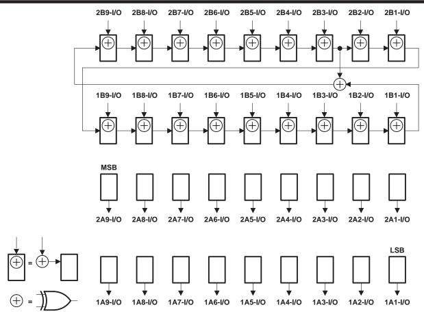
Figure 12. 18-Bit PSA/COUNT Configuration ( $1\overline{OEAB} = 2\overline{OEAB} = 1$ ,  $1\overline{OEBA} = 2\overline{OEBA} = 0$ )
