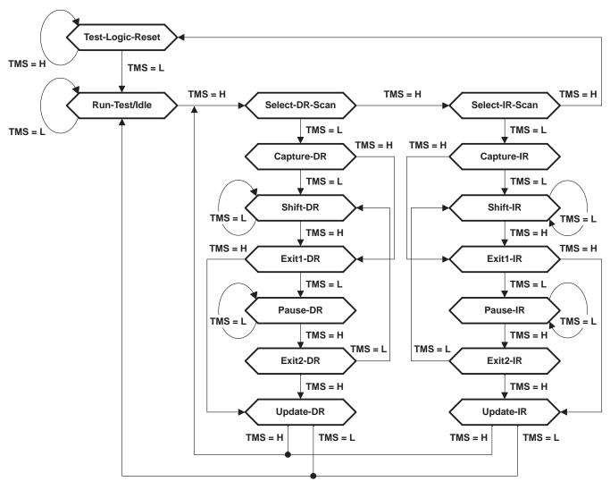
Figure 1. TAP-Controller State Diagram
