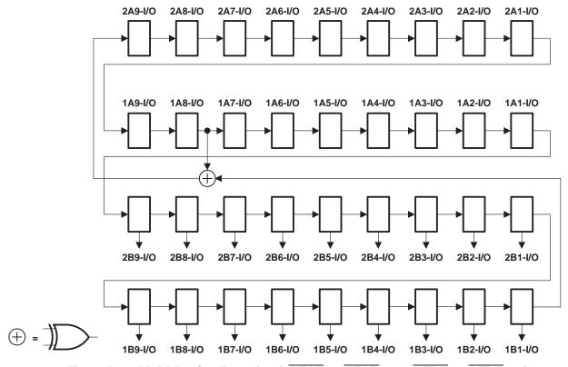
Figure 5. 36-Bit PRPG Configuration  $(1\overline{OEAB} = 2\overline{OEAB} = 0, 1\overline{OEBA} = 2\overline{OEBA} = 1)$
