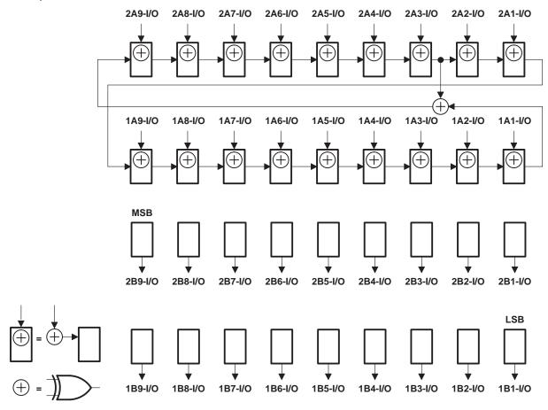
Figure 11. 18-Bit PSA/COUNT Configuration (1OEAB = 2OEAB = 0, 1OEBA = 2OEBA = 1)
