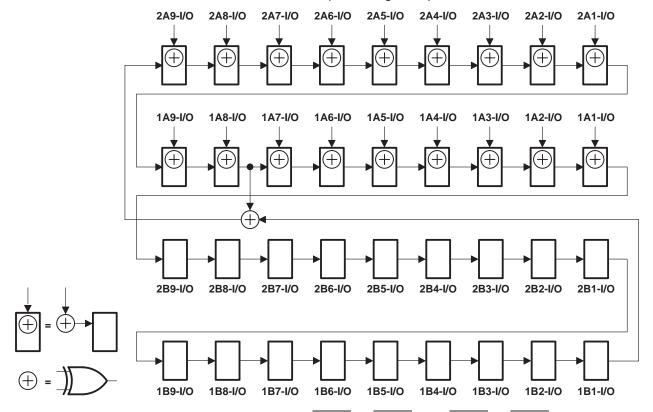
Figure 7. 36-Bit PSA Configuration  $(1\overline{OEAB} = 2\overline{OEAB} = 0, 1\overline{OEBA} = 2\overline{OEBA} = 1)$
