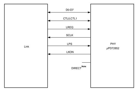
Note Clamping to VDD provides direct connection to Link.
