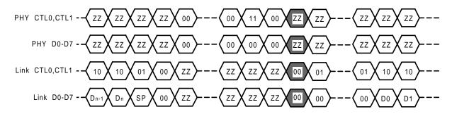
Note In case of packet transmission after Grant, before actual transmission, Hold does not need to be asserted.
