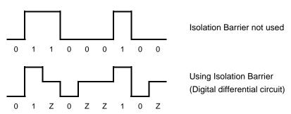
Figure 3-2. Waveforms of the Isolation Barrier
