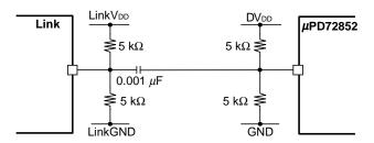
The Operating range of the power supply voltage is between 3.0 V and 3.45 V. Please refer to **IEEE1394a-2000 [5A.8.4]**.
