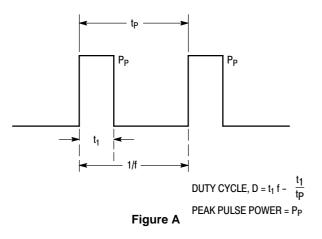
A train of periodical power pulses can be represented by the model shown in Figure A. Using the model and the device thermal response, the normalized effective transient thermal resistance of Figure 12 was calculated for various duty cycles.
