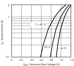
Source-Drain Diode Forward Voltage
