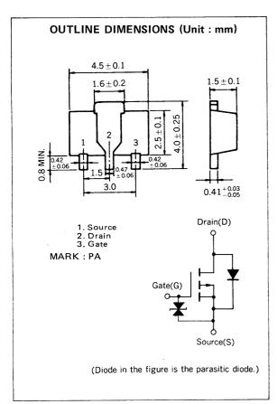
The 2SJ179, P-channel vertical type MOS FET, is a switching device which can be driven directly by the output of ICs having a 5 V power source.
