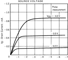
VDS-Drain to Source Voltage-V
