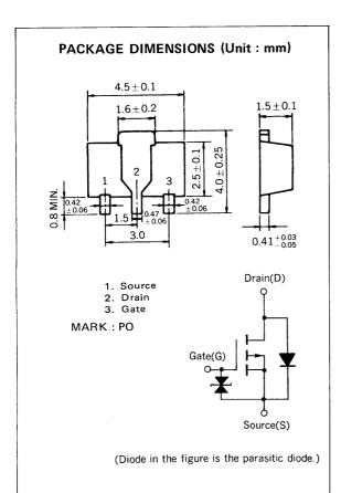
The 2SJ212, P-channel vertical type MOS FET, is a switching device which can be driven directly by the output of ICs having a 5 V power source.
