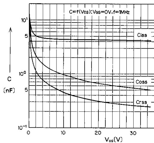
Typical Capacitance vs.  $V_{DS}$
