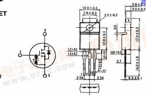
1. Gate 2. Drain 3. Source (Dimensions in mm)
