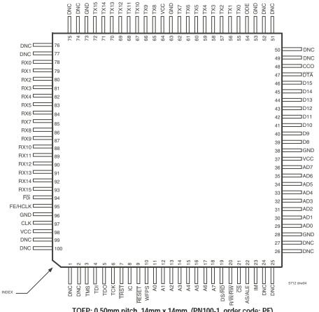
TQFP: 0.50mm pitch, 14mm x 14mm (PN100-1, order code: PF) TOP VIEW
