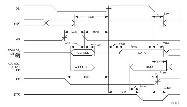
Figure 13. Multiplexed Bus Timing (Motorola Mode)
