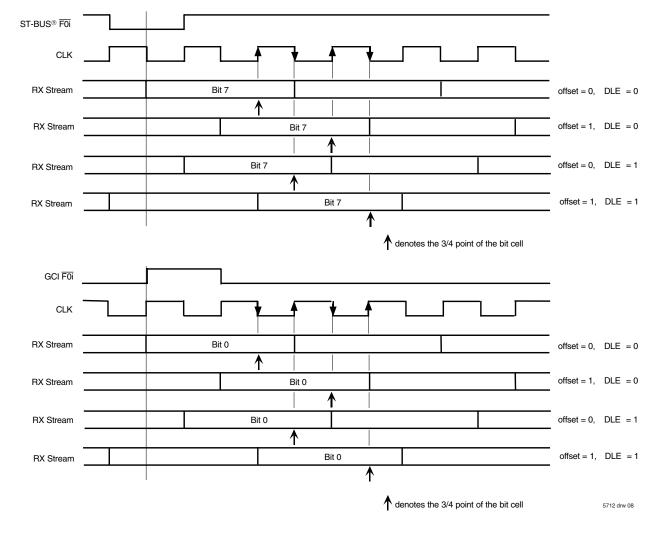
Figure 5. Examples for Input Offset Delay Timing
