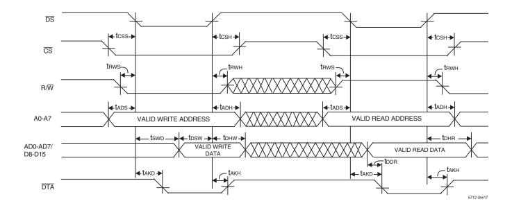
Figure 14. Motorola Non-Multiplexed Asyncronous Bus Timing
