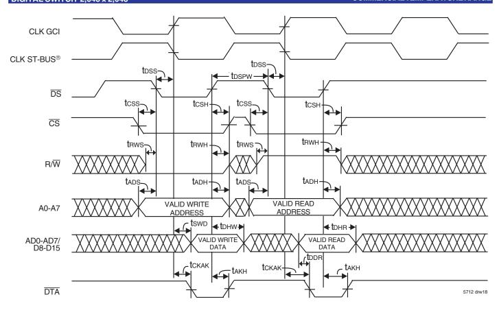
Figure 15. Motorola Non-Multiplexed Syncronous Bus Timing
