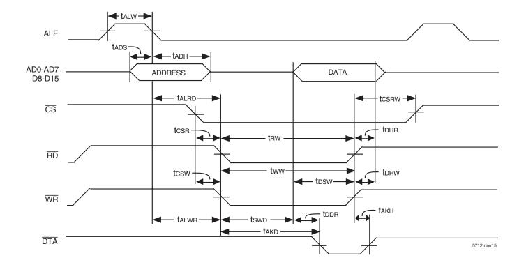
Figure 12. Multiplexed Bus Timing (Intel Mode)
