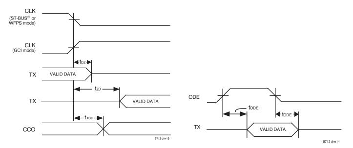
Figure 10. Serial Output and External Control
