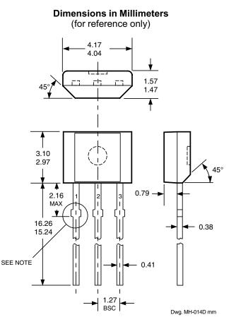
NOTES: 1. Tolerances on package height and width represent allowable mold offsets. Dimensions given are measured at the widest point (parting line).
