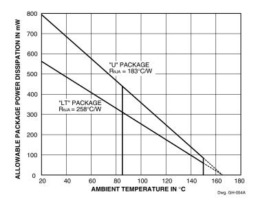
NOTE – Permitted duty cycle will be less than 100% at maximum ambient temperature with high supply voltages, i.e.,  $T_A \ge 140^{\circ}$ C,  $V_{CC} \ge 12$  V, and the "LT" package. The thermal shutdown circuitry does not protect the device from these stresses (see Internal Protective Features).
