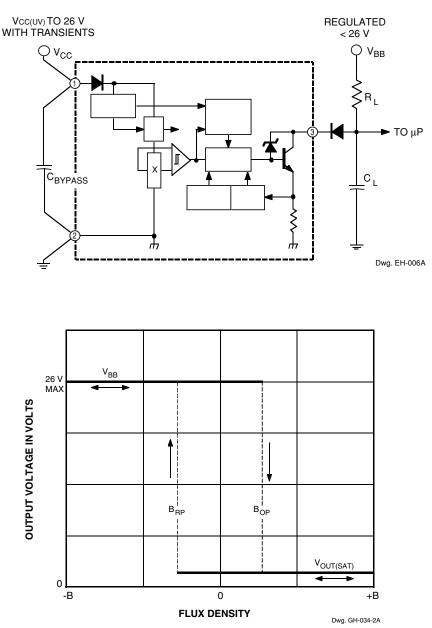
**Power Up Reset.** These devices are designed to power up with the output OFF without regard to any magnetic field applied. The output will remain OFF until the flux is reduced to below  $B_{RP}$  (S-N transition) and then  $B_{OP}$  is exceeded, depending on the turn-on state of the internal latches.
