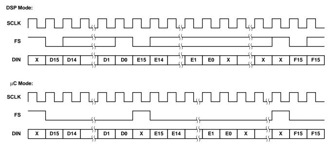
Difference between DSP mode (MODE = N.C. or 0) and  $\mu$ C (MODE = 1) mode:
