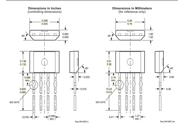
NOTES: 1. Tolerances on package height and width represent allowable mold offsets. Dimensions given are measured at the widest point (parting line).
