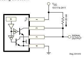
FIGURE 1 BIPOLAR DETECTOR
