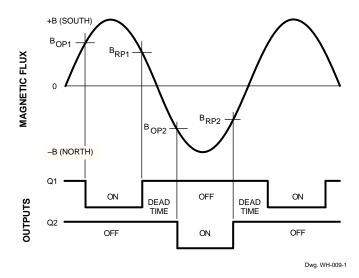
FIGURE 2 ZERO-CROSSING DETECTION
