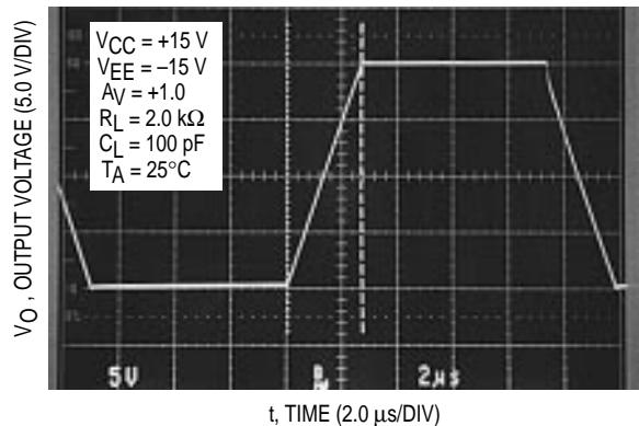
**Figure 32. Noninverting Amplifier Overshoot**
