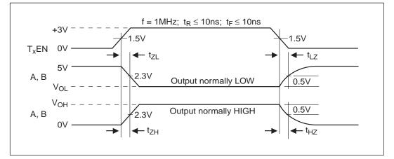
Figure 6. Driver Enable and Disable Times
