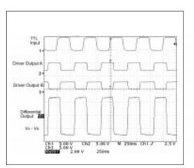
Figure 10. Typical RS-485 Driver Output
