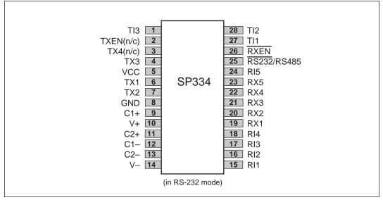
Figure 11. SP334 Pinout
