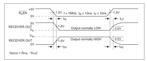
Figure 8. Receiver Enable and Disable Times
