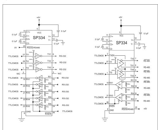
Figure 12. Typical Operating Circuit
