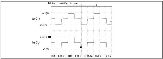
Figure 17. Charge Pump Waveforms
