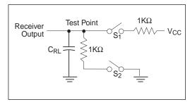
Figure 2. Receiver Timing Test Load Circuit
