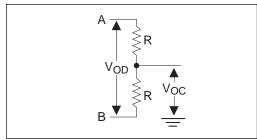
Figure 1. Driver DC Test Load Circuit
