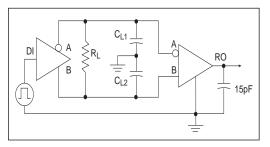
Figure 3a. Driver/Receiver Timing Test Circuit
