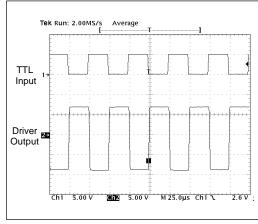
Figure 9. Typical RS-232 Driver Output
