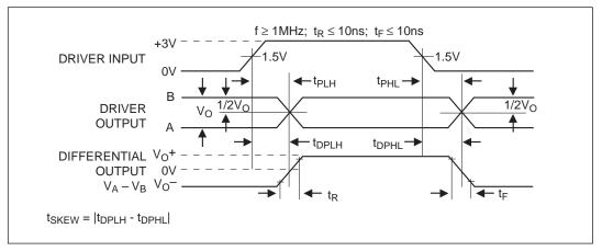
Figure 5. Driver Propagation Delays
