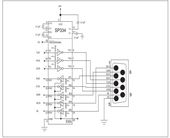
Figure 18. SP334 Configuration to a DB-9 Serial Port
