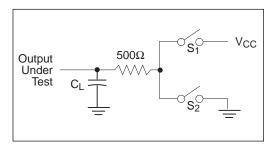
Figure 4. Driver Timing Test Load #2 Circuit
