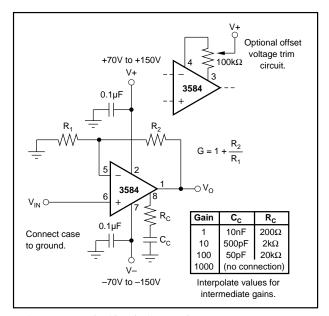
FIGURE 1. Basic Circuit Connections.
