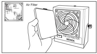
Figure 5: Replace the filter.
