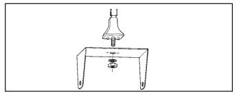
Figure 4: Installing The Extractor to Swing Arm
