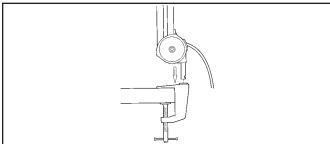
Figure 3: Installing Swing Arm on workbench
