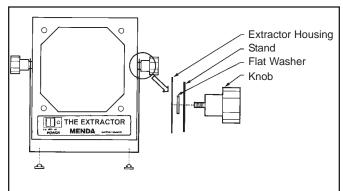
Figure 2: Installing stand assembly
