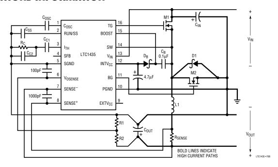
Figure 8. LTC1435 Layout Diagram
