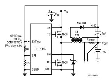
Figure 4a. Secondary Output Loop and EXTV<sub>CC</sub> Connection
