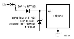
Figure 7. Automotive Application Protection
