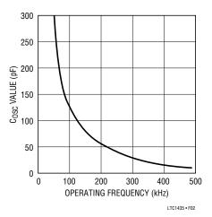
Figure 2. Timing Capacitor Value
