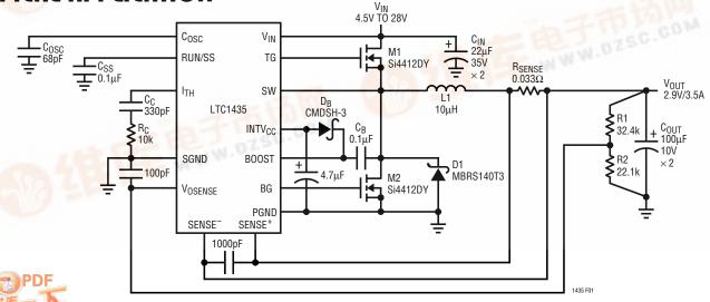
Figure 1. High Efficiency Step-Down Converter
