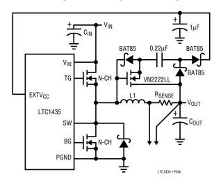
Figure 4b. Capacitive Charge Pump for EXTV<sub>CC</sub>
