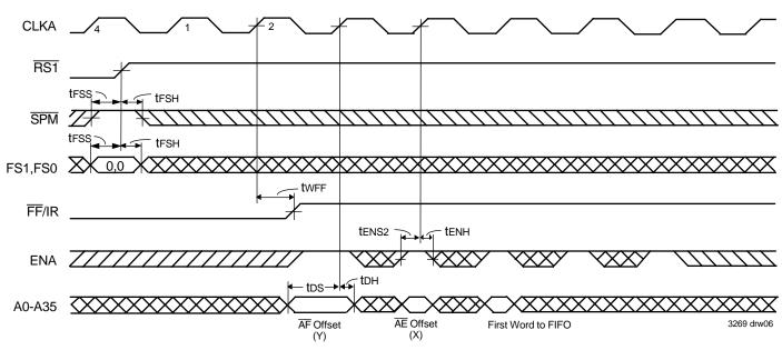
1.  $\overline{\text{CSA}}$  = LOW, W/ $\overline{\text{R}}$ A = HIGH, MBA = LOW. It is not necessary to program offset register on consecutive clock cycles.
