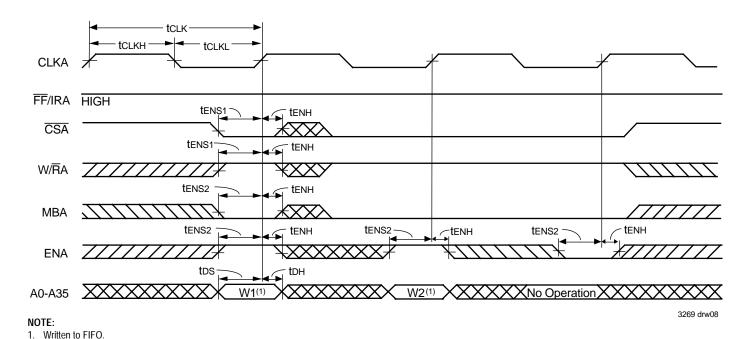
Figure 7. Port A Write Cycle Timing for FIFO (IDT Standard and FWFT Modes)
