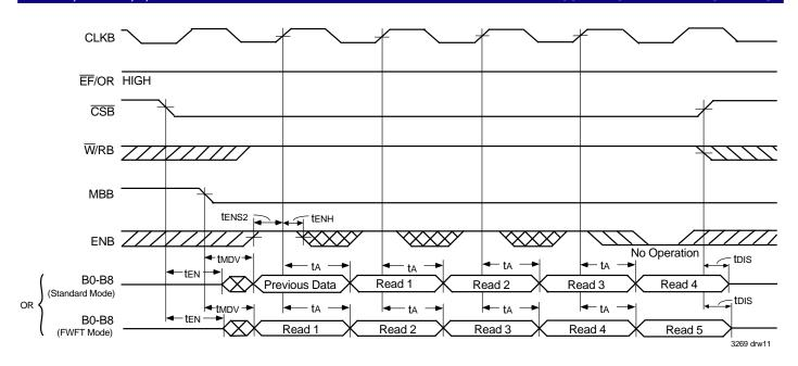
1. Unused bytes B9-B17, B18-B26, and B27-B35 are indeterminate.
