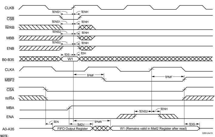
1. If Port B is configured for word size, data can be written to the Mail2 Register using B0-B17 (B18-B35 are don't care inputs). In this first case A0-A17 will have valid data (A18-A35 will be indeterminate). If Port B is configured for byte size, data can be written to the Mail2 Register using B0-B8 (B9-B35 are don't care inputs). In this second case, A0-A8 will have valid data (A9-A35 will be indeterminate).
