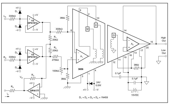
FIGURE 7. Driven Right-Leg Amplifier.
