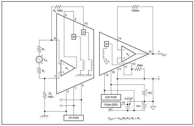
FIGURE 11. Differential Input, Floating Source.
