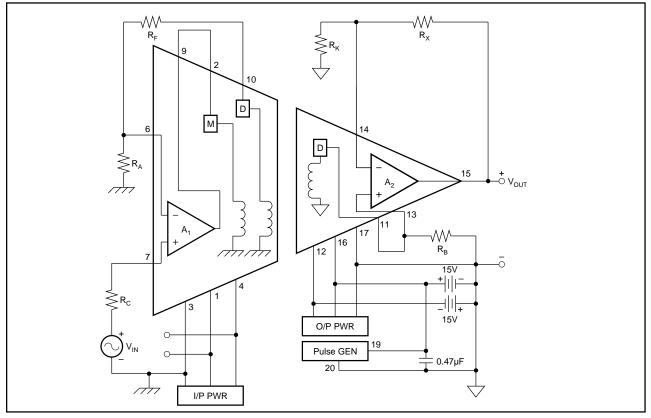
FIGURE 3. Power: Two-Port, Dual Supply; Signal: Noninverting Gain.
