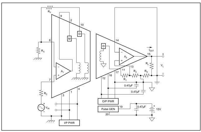
FIGURE 8. Bipolar Current Output.
