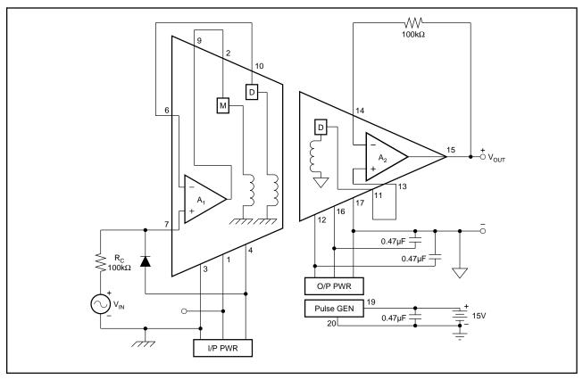
FIGURE 2. Power: Three-Port Isolation; Signal: Unity-Gain Noninverting.
