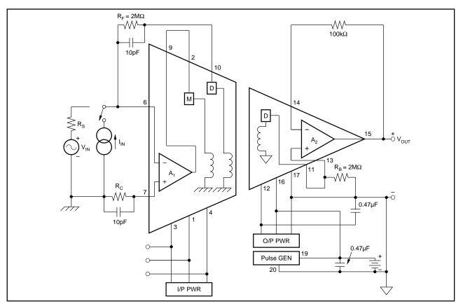
FIGURE 4. Power: Two-Port, Single Supply; Signal: Inverting Gains.
