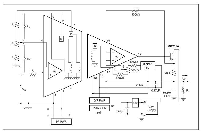
FIGURE 10. Isolated 4mA to 20mA  $\rm I_{OUT}$
