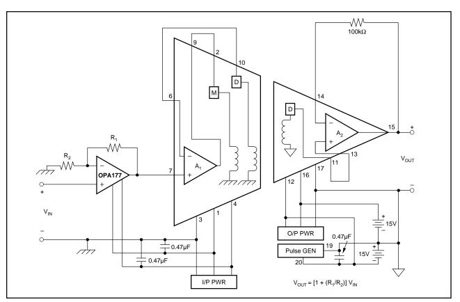
FIGURE 13. Isolator for Low-Level Signals.
