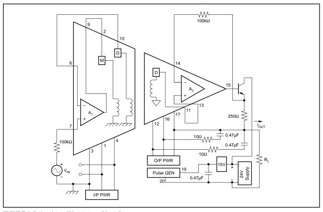
FIGURE 9. Isolated 1 to  $5V_{_{\mbox{\footnotesize IN}}}\!/\,4mA$  to 20mA  $I_{_{\mbox{\footnotesize OUT}}}\!.$
