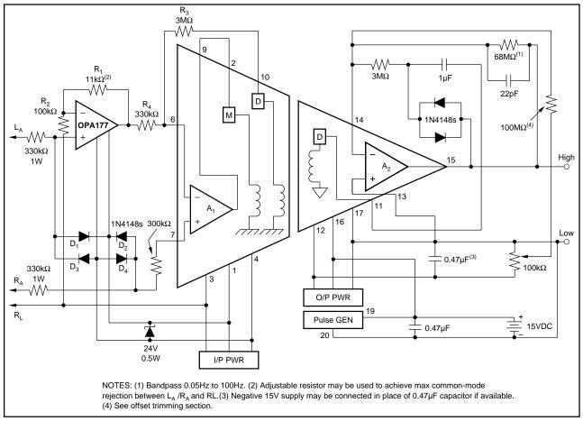
FIGURE 6. ECG Amplifier.
