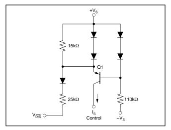
FIGURE 13. Simplified Disable Control Circuit.
