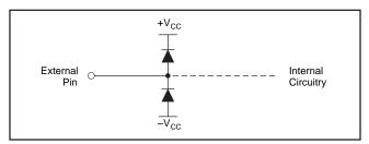
FIGURE 15. Internal ESD Protection.
