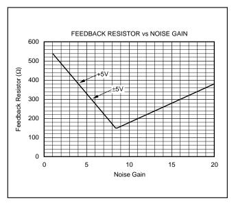
FIGURE 10. Recommended Feedback Resistor vs Noise Gain.
