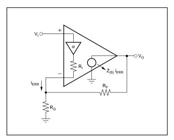
FIGURE 9. Current Feedback Transfer Function Analysis Circuit.
