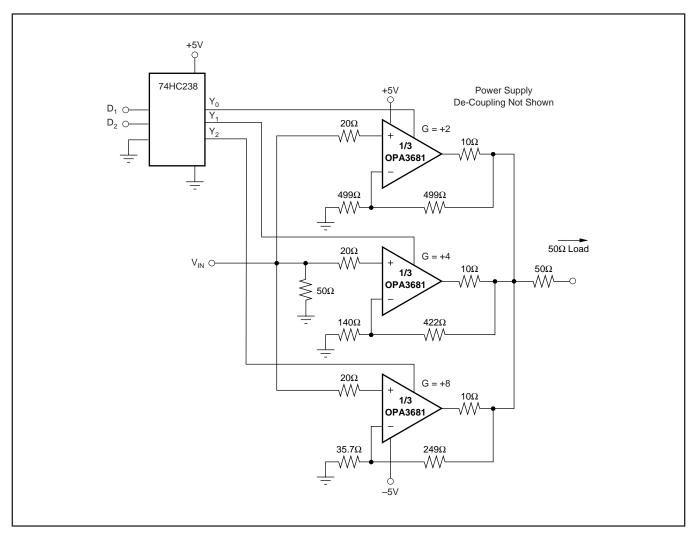
FIGURE 8. Wideband Programmable Gain.
