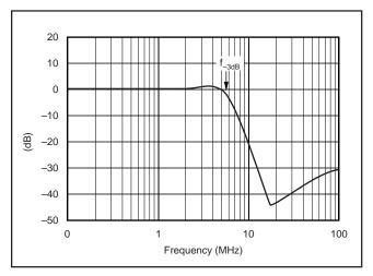
FIGURE 6. DAC Reconstruction Filter Response.
