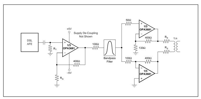
FIGURE 7. Single-to-Differential xDSL Line Driver.
