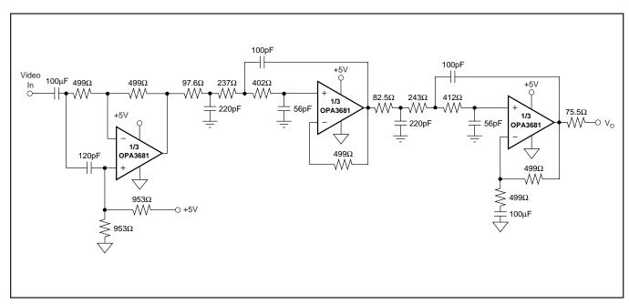
FIGURE 5. Filter Schematic.
