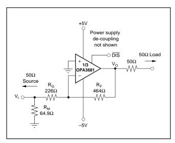
FIGURE 11. Inverting Gain of -2 with Impedance Matching.
