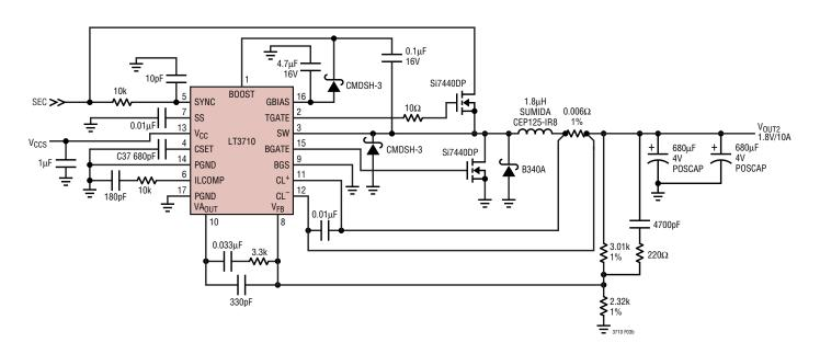
Figure 3b. 36V to 72V DC to 3.3V/10A and 1.8V/10A Dual Output Isolated Power Supply (Part 2 of 2, See Previous Page)
