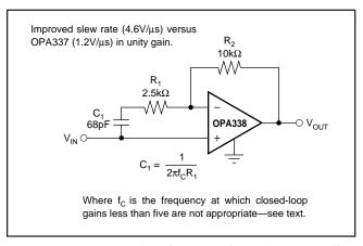
FIGURE 3. Compensation of OPA338 for Unity-Gain Buffer.
