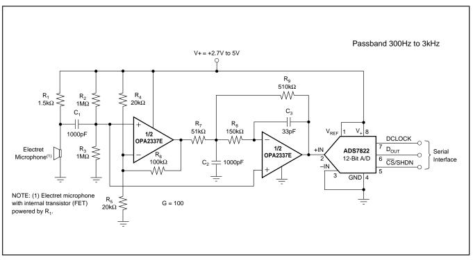
FIGURE 6. Low Power, Single-Supply, Speech Bandpass Filtered Data Acquisition System.
