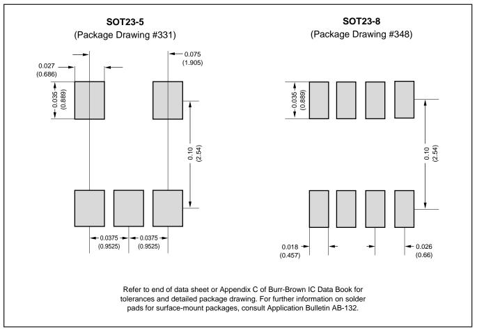
FIGURE 7. Recommended SOT23-5 and SOT23-8 Solder Footprints.
