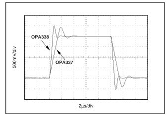
FIGURE 5. G = 2, Slew-Rate Comparison of OPA338 and OPA337.
