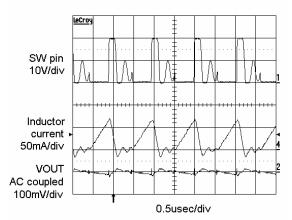
Switching Waveform VIN = 4.2V,  $I_{LED} = 4mA$
