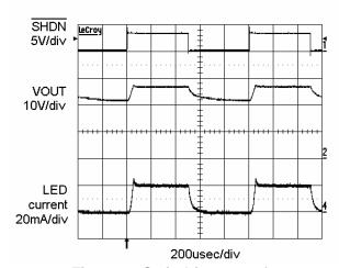
Figure 1. Switching waveform with 1kHz PWM on SHDN\*
