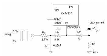
Figure 2. Circuit for filtered PWM signal
