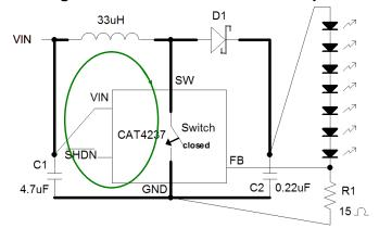
Figure 4. Open-switch current loop
