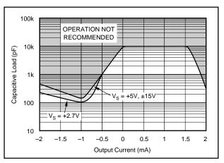
FIGURE 1. Stability-Capacitive Load vs Output Current.
