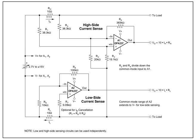
FIGURE 2. Low and High-Side Battery Current Sensing.
