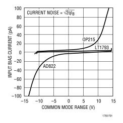
Figure 1. Comparison of LT1793, OP215, and AD822 Input Bias Current vs Common Mode Range
