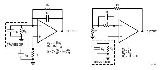
Figure 4. Inverting and Noninverting Gain Configurations
