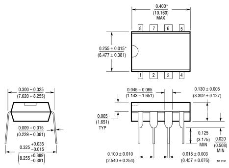
\*THESE DIMENSIONS DO NOT INCLUDE MOLD FLASH OR PROTRUSIONS. MOLD FLASH OR PROTRUSIONS SHALL NOT EXCEED 0.010 INCH (0.254mm) **PACKAGE DESCRIPTION** Dimensions in inches (millimeters) unless otherwise noted.
