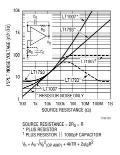
Figure 3. Comparison of LT1793 and LT1007 Total Output 1kHz Voltage Noise vs Source Resistance
