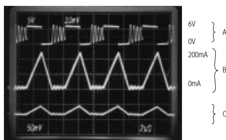
SWITCHING WAVEFORMS, DISCONTINUOUS CONDUCTION
