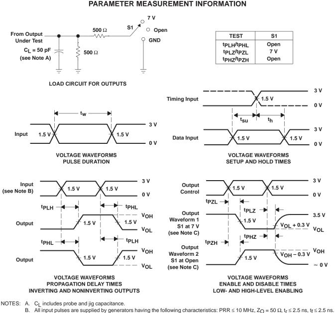
All input pulses are supplied by generators having the following characteristics: PRR ≤ 10 MH2, ∠O = 50 Ω, t<sub>r</sub> ≤ 2.5 ns, t<sub>f</sub> ≤ 2.5 ns
