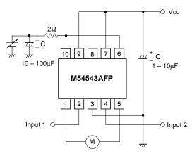
3) When Vcc is used as a variable power supply and Vcc' is used as a fixed power supply
