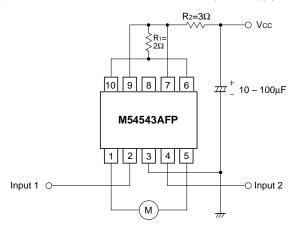
2) When Vcc is used as a fixed power supply and Vcc' is used as a variable power supply
