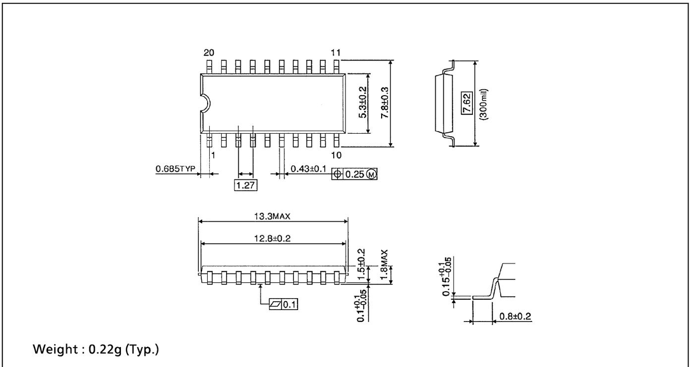
SOP 20PIN (300mil BODY) PACKAGE DIMENSIONS (SOL20-P-300-1.27)
