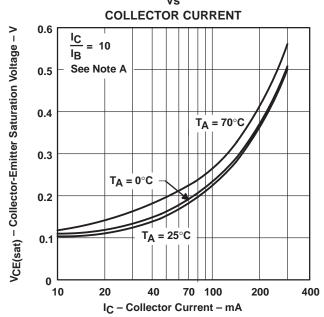
NOTE A: These parameters must be measured using pulse techniques,  $t_{\text{W}}=300~\mu\text{s},$  duty cycle  $\leq 2\%.$
