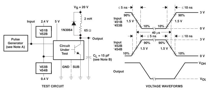
NOTES: A. The pulse generator has the following characteristics: PRR  $\leq$  12.5 kHz,  $Z_O$  = 50  $\Omega$ .
