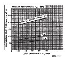
Fig. 6 — Typical propagation delay time vs. load capacitance (SET to  $\overline{Q}$  or RESET to Q.
