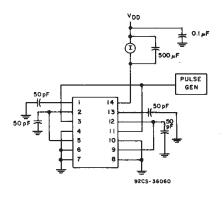
Fig. 13—Dynamic power dissipation test circuit.
