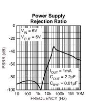
**Power Supply Rejection Ratio** 0 = 6\ 5\ -20 PSRR (dB) -40 -60 = 10mA I<sub>OUT</sub> -80  $C_{OUT} = 2.2 \mu F$  $C_{BYP} = 0.01 \mu F$ -100 , 10 1k 10k 100k 1M 10M 100 FREQUENCY (Hz)
