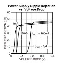
Power Supply Ripple Rejection vs. Voltage Drop
