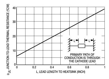
Figure 1. Typical Thermal Resistance
