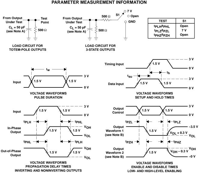
NOTES: A. C<sub>1</sub> includes probe and jig capacitance.
