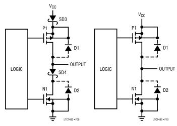
Figure 9. LTC1483 Output Stage
