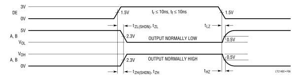
Figure 6. Driver Enable and Disable Times
