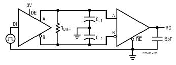
Figure 3. Driver/Receiver Timing Test Circuit
