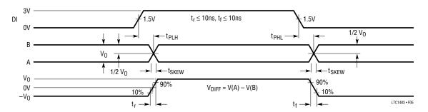
Figure 5. Driver Propagation Delays
