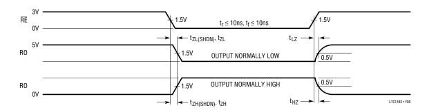
Figure 8. Receiver Enable and Disable Times
