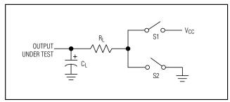
Figure 4. Driver Enable/Disable Timing Test Load
