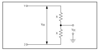
Figure 1. Driver DC Test Circuit
