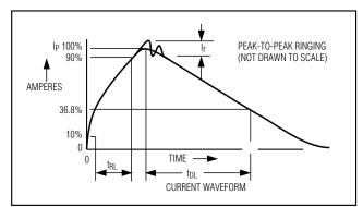
Figure 6b. Human Body Model Current Waveform
