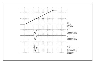
Figure 11. Differential Power-Up Glitch (0.1V/µs)
