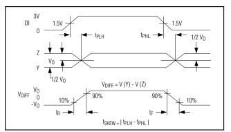
Figure 3. Driver Propagation Delays
