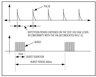
Figure 8. General Graph of a Fast Transient Burst
