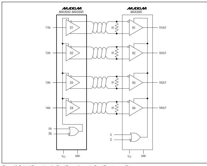
Figure 13. Typical Connection of a Quad Transmitter and a Quad Receiver as a Pair
