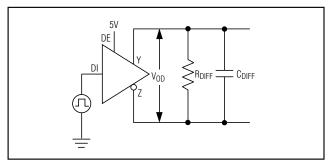
Figure 2. Driver Timing Test Circuit
