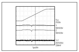
Figure 12. Differential Power-Up Glitch (1V/µs)
