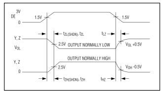
Figure 5. Driver Enable and Disable Times
