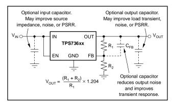
Figure 32. Typical Application Circuit for Adjustable-Voltage Versions
