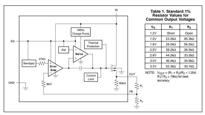
Figure 2. Adjustable Voltage Version
