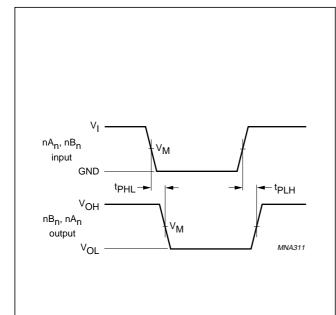
Fig.5 The input  $nA_n$ ,  $nB_n$  to output  $nB_n$ ,  $nA_n$  propagation delay times.
