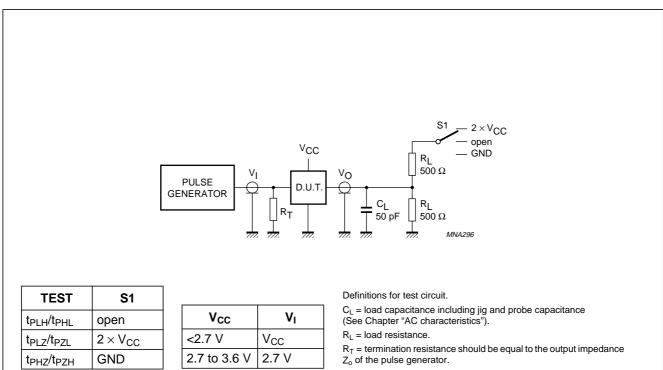
Fig.8 Load circuitry for switching times.
