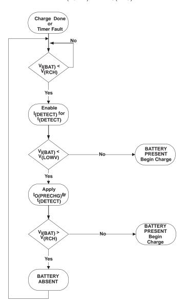
Figure 7. Battery Absent Detection
