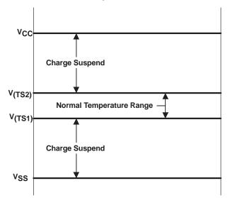
Figure 6. TS Pin Thresholds
