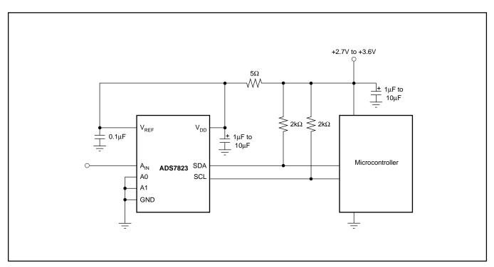
FIGURE 1. Simplified I/O of the ADS7823.
