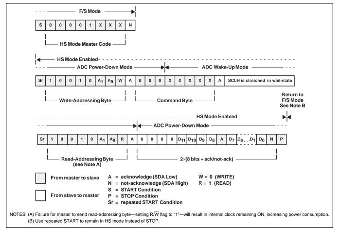
FIGURE 4. Typical Read Sequence in HS Mode.
