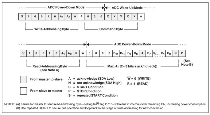
FIGURE 3. Typical Read Sequence in F/S Mode.
