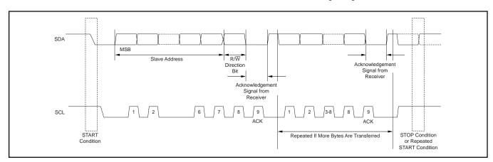
FIGURE 2. Basic Operation of the ADS7823.
